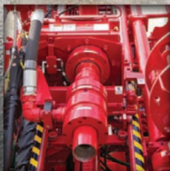
TOP-HEAD DRIVE Multiple options available including combination side inlet/discharge swivel mounted to floating shaft.
