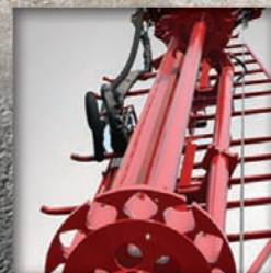
PIPE CAROUSEL Hydraulic pipe arm or available pipe carousel significantly improves safety, reliability and production efficiency.
